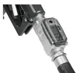
Light weight aluminum turbine meter. Flow range of 3 to 30 GPM (10 to 100 LPM). Powered by two AAA batteries that are easy to replace. Factory calibrated for fuel. Typical accuracy of +/- 2.5 (accuracy can vary to +/- 5%.
