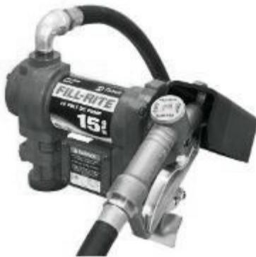
This standard duty 1/4 HP explosion proof UL listed pump can pump Up to 15 GPM. Has a 2" threaded base for tank mounting, cast bronze rotor with bronze rotary vanes, and built in strainer. 2 Year warranty.
