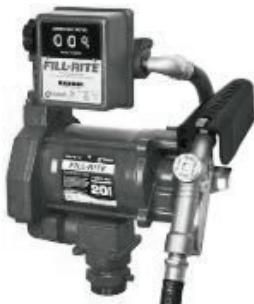
Heavy duty UL listed explosion proof 1/3 HP motor. 807C Meter. Heavy duty switch, thermal overload protection and junction box. Carbon vanes and ceramic/carbon seals. Integral check valve with pressure relief on outlet side. Easy removable strainer, automatic bypass valve, 2" threaded bung for tank openings. 2 Year warranty.
