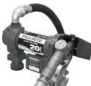
This contractor grade pump with explosion proof UL approved motor pumps Up to 20 GPM. Built using heavy duty cast iron this pump has a 2" threaded base for tank mounting, cast bronze rotor with bronze rotary vanes, and built in strainer. 2 Year warranty.
