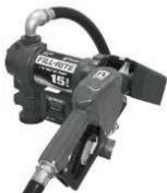
This Standard duty pump has a 1/6 HP Explosion proof motor and pumps UP to 15 GPM. Pumps has a 2" threaded base for tank openings, carbon vanes, check valve, pressure relief valve, and strainer. 2 Year warranty.
